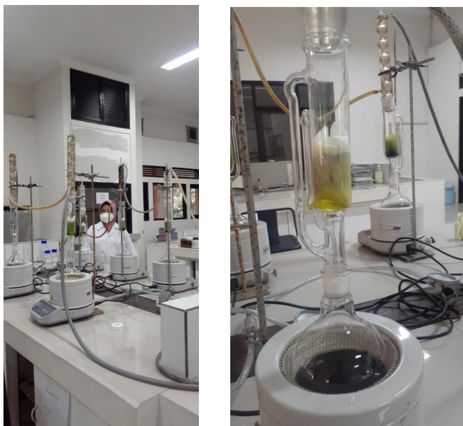
Figure 2. Moringa Leaf and Powder Soxhlet Tool Set
